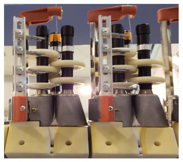
Chines Patent "Single driven and Tension controlled Texturing Unit FK6 (patented) for highest quality textured yarn".
